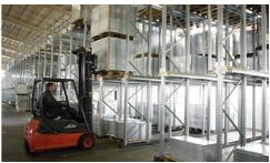
Drive-in racking eliminates the need for loading and picking aisles. The lift truck positions pallets on front-to-back rails, allowing rows to be stacked next to each other. Dexion drive-in racking provides a safe and efficient equivalent of block stacking for loads which are too fragile or unstable to be stacked on top of each other.
