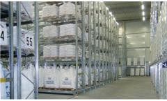
The electronically controlled MOVO heavy duty mobile pallet racking system runs on embedded rails and can carry bay loads of up to 24 tons at racking heights of up to 12 metres, with runs up to 90m possible.
