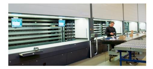
Automatic Storage Machines are computer-controlled storage and transfer systems that can significantly improve the efficiency of product storage and picking.
