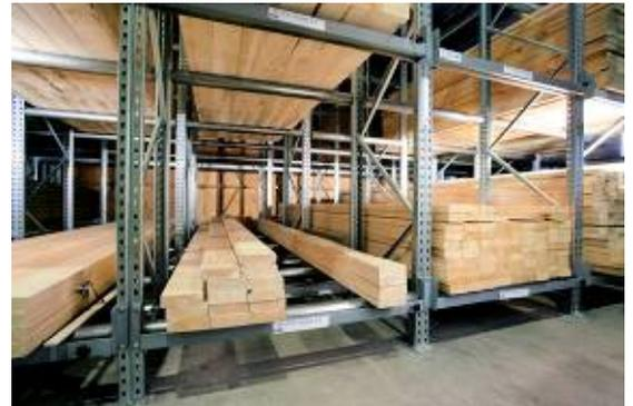
Once the goods have been placed into the storage locations the rollers can be locked for safety, allowing individual pieces to be removed one at a time.
