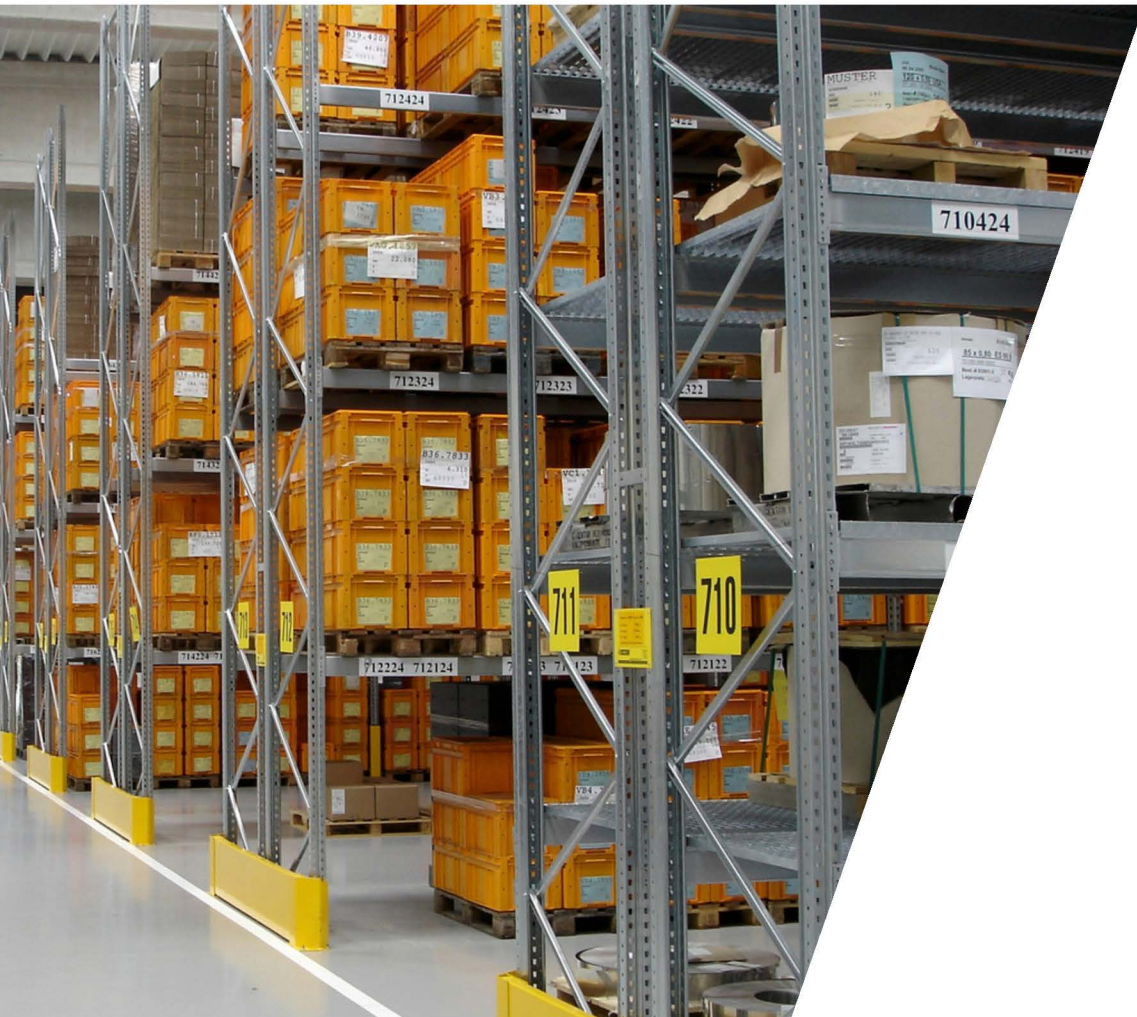
Standard Pallet Racking
